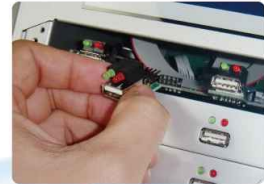
Easier port module exchange to reduce maintenance effort.
